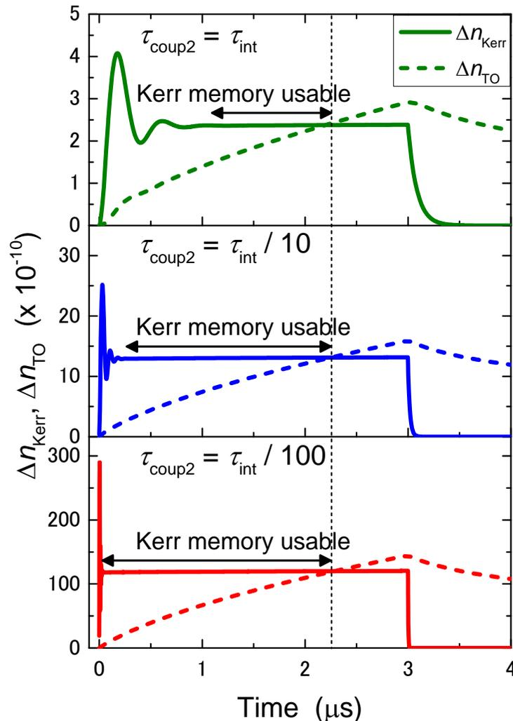
□ Refractive index change caused by Kerr and TO effects in 4-port system.
