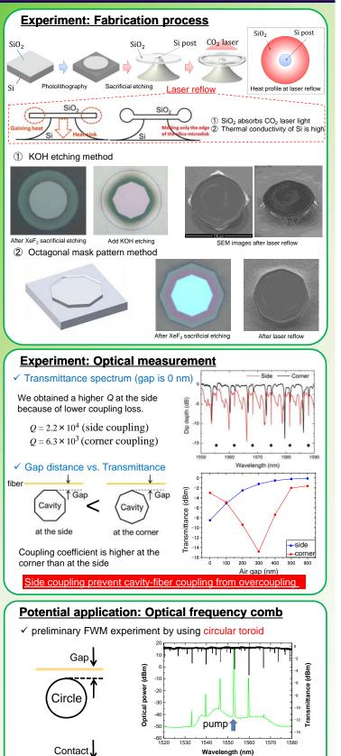
By performing similar experiment with polygonal cavity, we may enable the demonstration of the robust micro-sized frequency comb generator.
