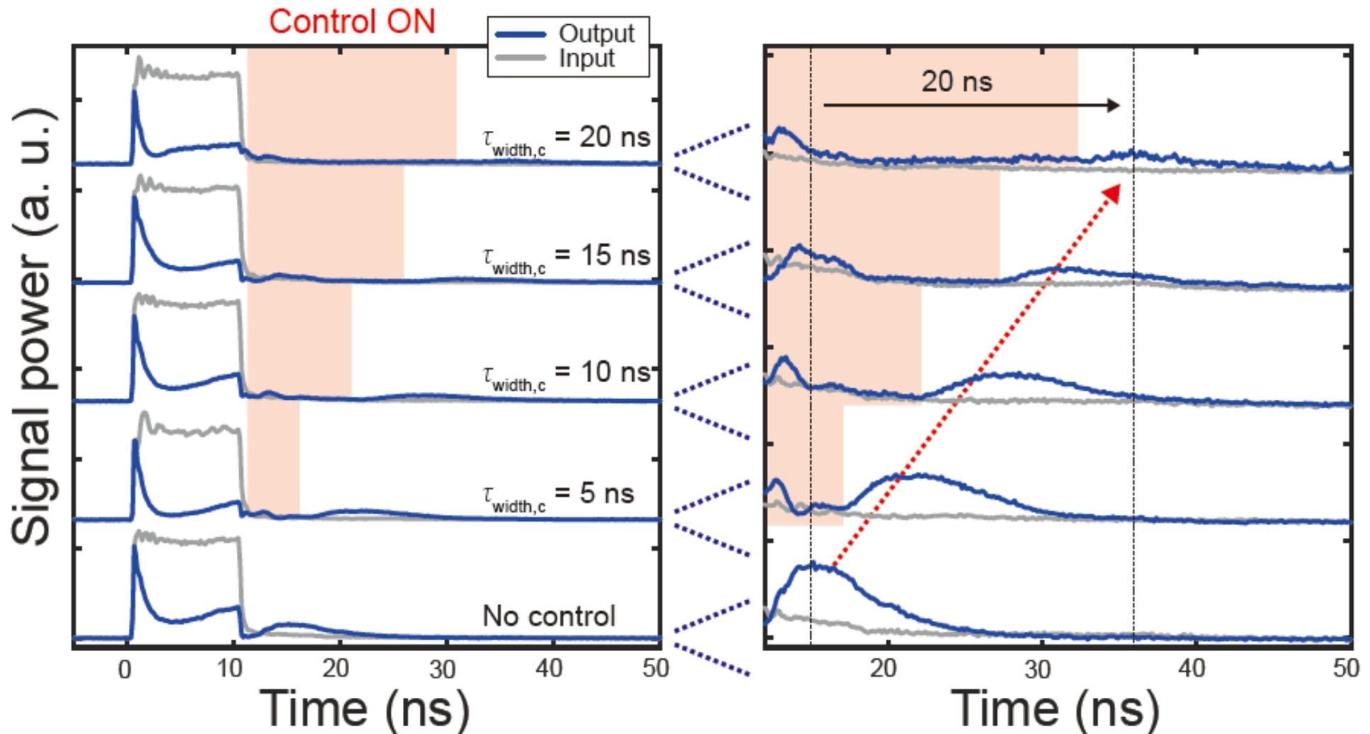
**All-optical tunable buffering / 10-ns pulse buffered for 20 ns**
