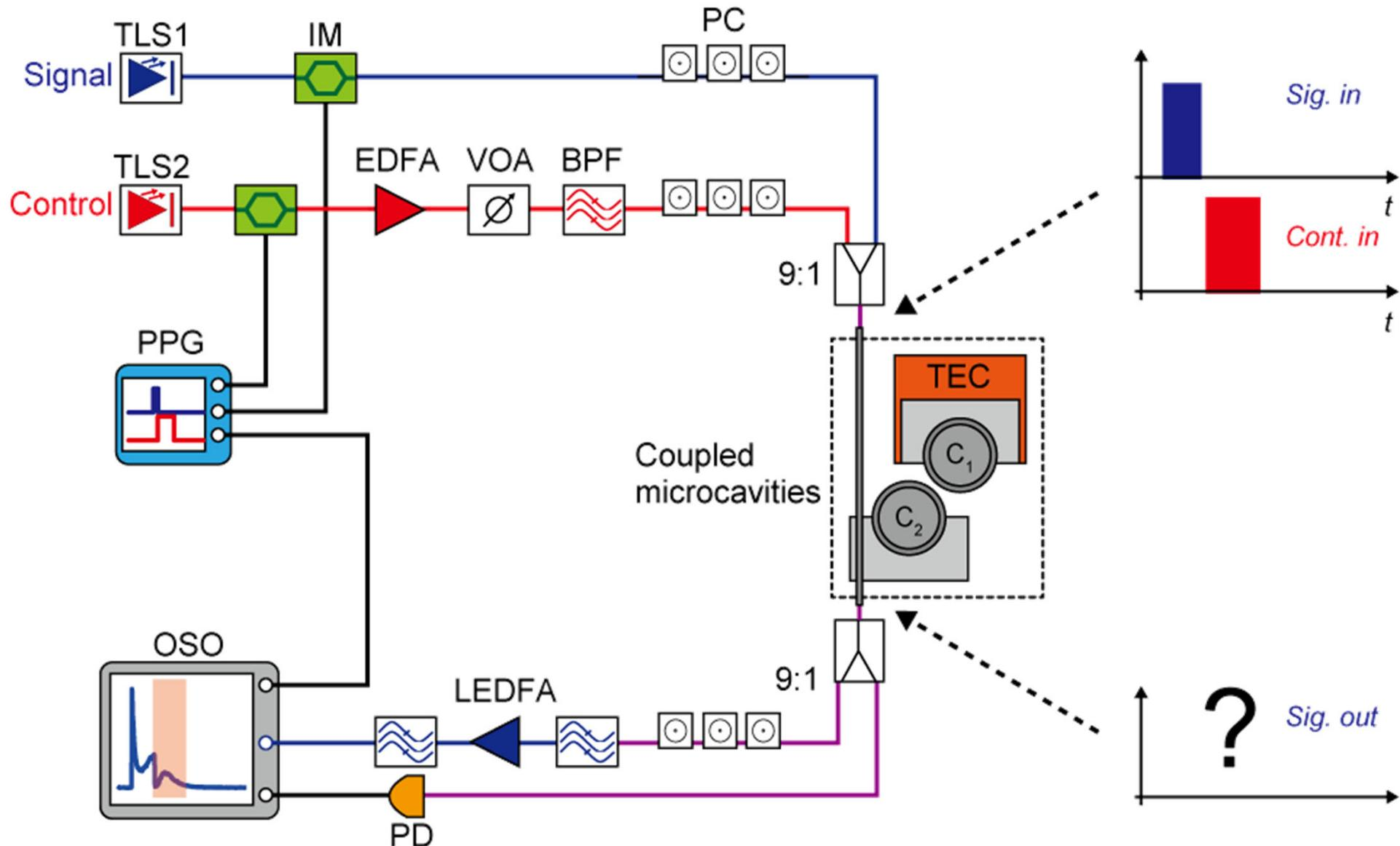
**TLS:** Tunable laser source / **IM:** Intensity modulator / **EDFA:** Erbium-doped fiber amplifier
