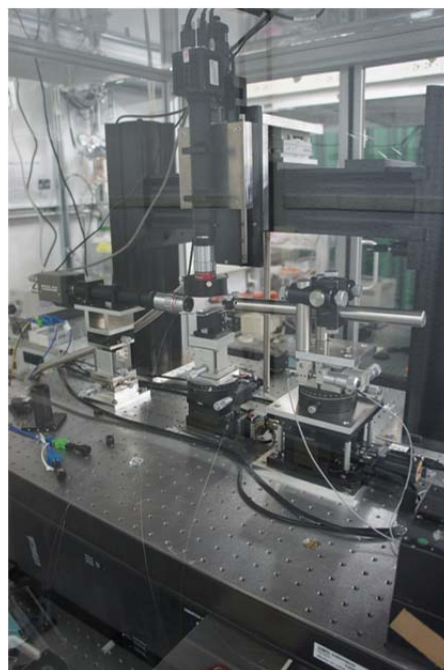
Fig. 2. Photograph of fiber-taper coupling setup.
