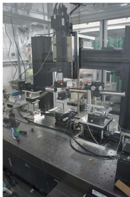
Fig. 2. Photograph of fiber-taper coupling setup.
