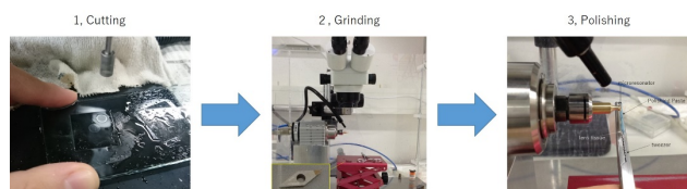
Fig. 1 : Flow chart of crystalline microresonator fabrication process .
