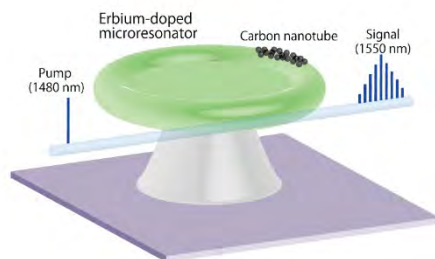
Fig. 1. A schematic illustration of a mode-locked laser with CNTs and an Er-doped microresonator.
