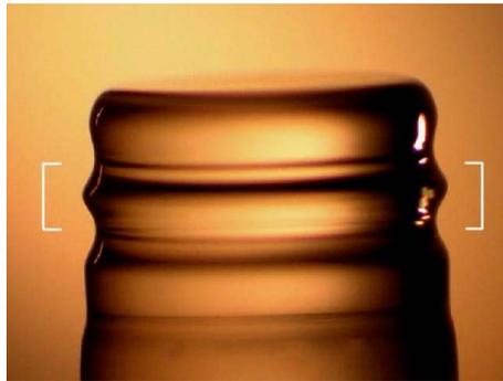
Fig.1.5. microscope image of  $\text{CaF}_2$  crystalline microcavity [I. S. Grudinin, V. S. Ilchenko, and L. Maleki, “Ultra-high optical  $Q$  factors of crystalline resonators in the linear regime,” *Phys. Rev. A* 74, 063,806 (2006).].
