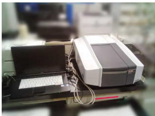
Fig. 4.3: UV-vis absorption spectroscopy I used. This equipment is located in 中央試験所
