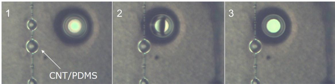
Fig. 5.1: These three pictures represent the method of coating CNT/PDMS to the edge of microtoroid.
