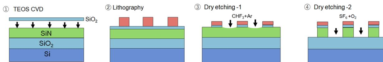
Fig.4.4 Schematic illustration of CE with TEOS mask.
