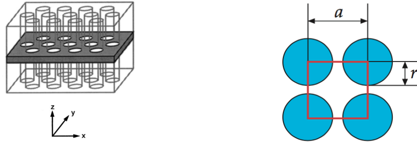
Figure (2.3): 2D PhC structure [Shanhui Fan Steven G. Johnson Pierre R. Villeneuve and J.D Joannopoulos. “Linear waveguides in photonic-crystals slabs”. In: Physical Review B 62 (2000).]
