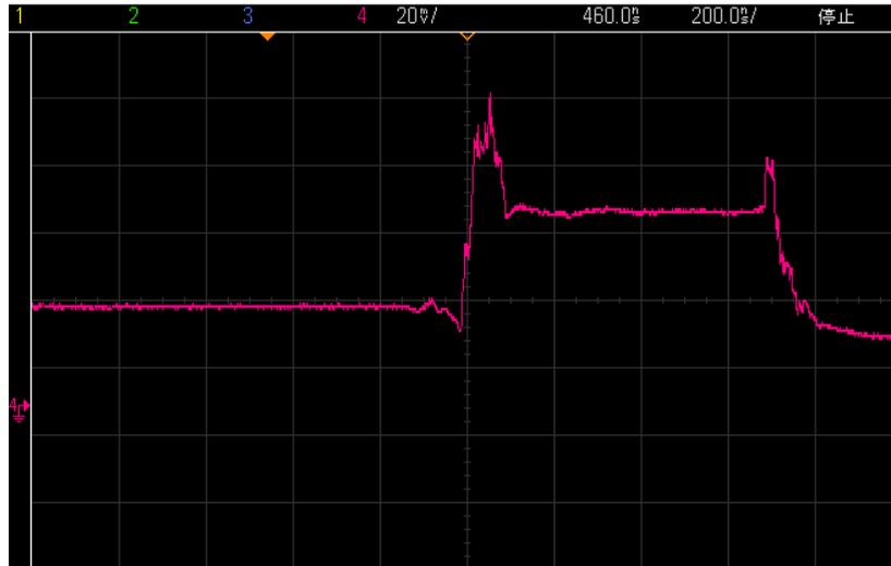
Fig. 3.14. Screen shot of oscilloscope with a 600 ns soliton step.
