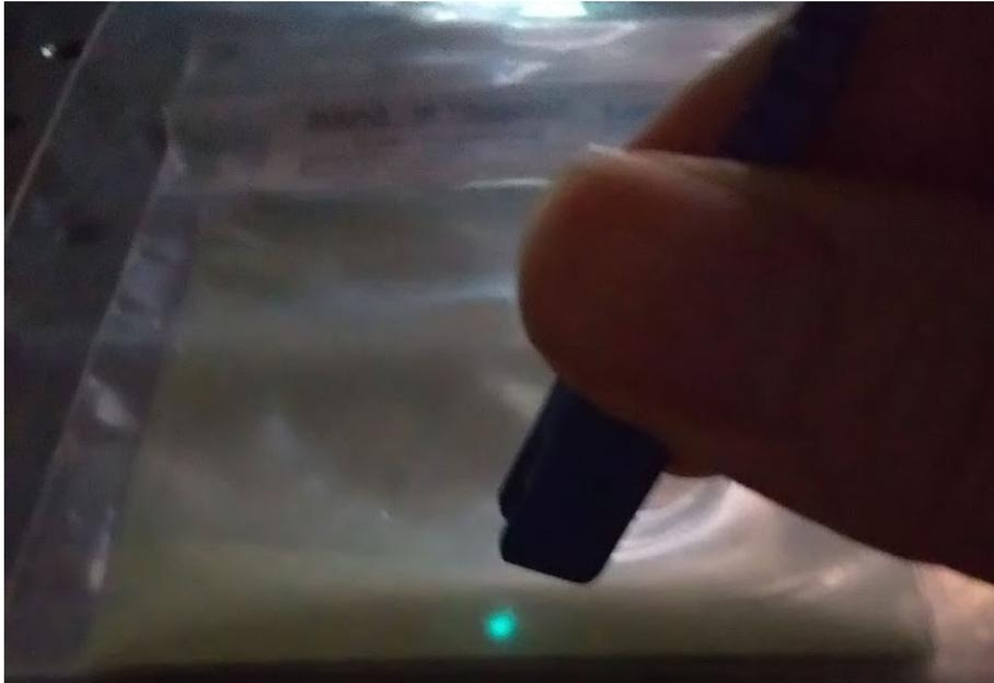
Fig. 3.6: The image of a phosphor illuminated with light of a communication wavelength.
