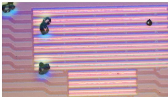
Fig. 4.5: This is a photonic crystal waveguide after coating using PDMS. There are no cracks on the surface. The black objects are phosphor particles.
