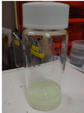
Fig. 3.7: PDMS solution: The phosphor remains in the solution.
