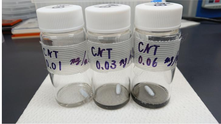
Fig.5.7 The phot of the mixture of PDMS and CNTs fabricated. No agglomeration was observed even though the mixture was made with different concentrations.
