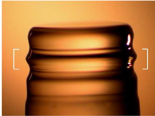
Fig. 1.3 Photo image of  $\text{CaF}_2$  crystalline microcavity.
