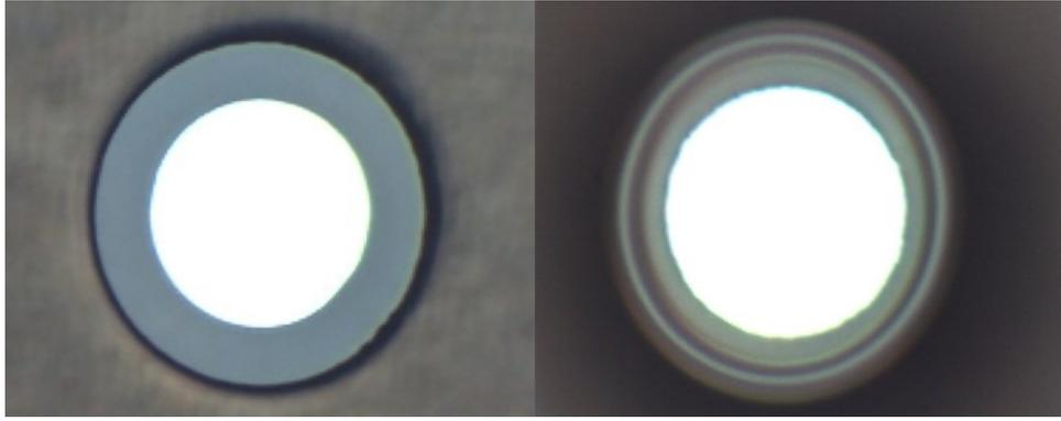
Fig. 5.6: Microscope images of a disk resonator (left) and a toroid resonator (right).
