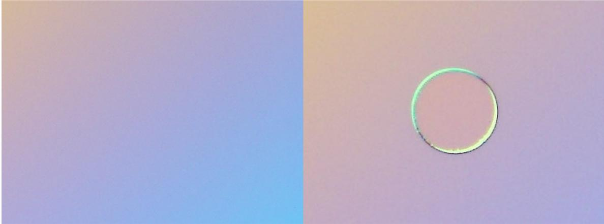
Fig. 5.4: Microscope images of a silica film (left) and a photoresist pattern transferred by photolithography.
