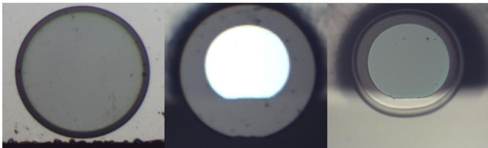
Fig. 5.8: Microscope images of a silica substrate after dicing (left), dry etching (middle), and CO<sub>2</sub> laser reflow (right).
