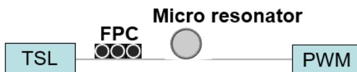
Fig3-8 diagram of the experimental setup for measurement of quality factor.
