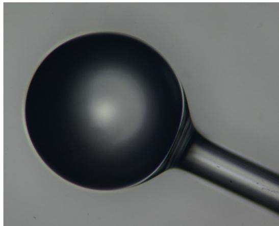
Fig. 5.6 Photo of a large size microsphere resonator.
