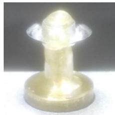
Fig. 3.2: MgF<sub>2</sub> microresonator I fabricate
