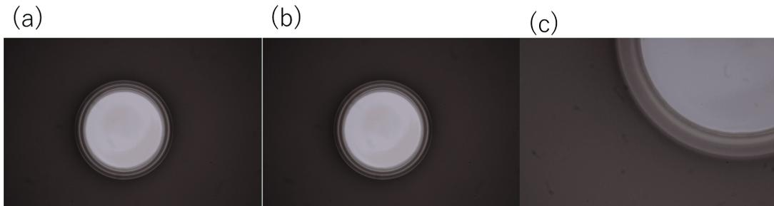
Fig. 4.3: (a)High Q factor microtoroid before transferring graphene observed with optical microscope. (b)The microtoroid after transferring. (c)A picture of microtoroid which enlarged the place where graphene was transferred to.
