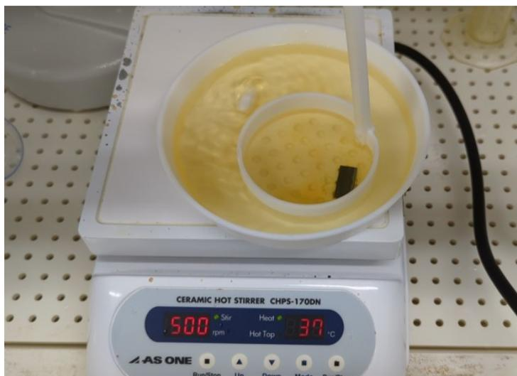
Fig.1.5: HNA etching:the yellow color of the solution is derived from NO<sub>2</sub>
