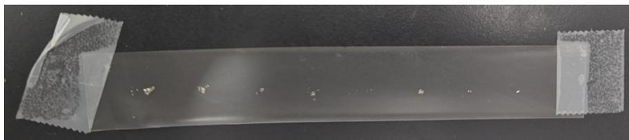
Fig.4.8: Graphene flakes on scotch tape.
